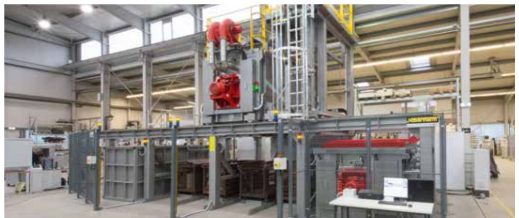
Drop-bottom furnace plant for aluminum
